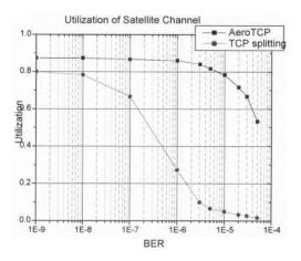
Figure 7 Utilization for different bit error rates
