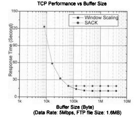
Figure 4. TCP performance with different buffer size
