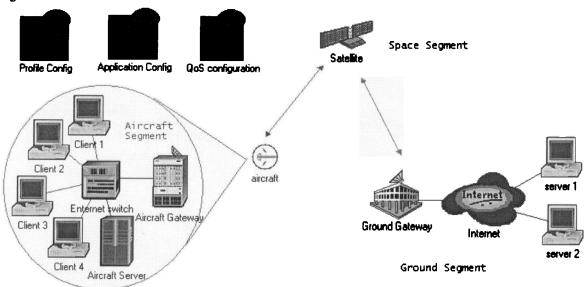
Figure 2 Experiment setup for End-to-end TCP solutions
