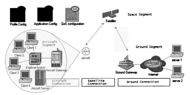
Figure 5 TCP Splitting protocol for Aeronautical Satellite Networks
