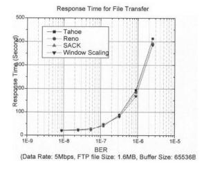
Figure 3. TCP performance for satellite link (1.6MB)
