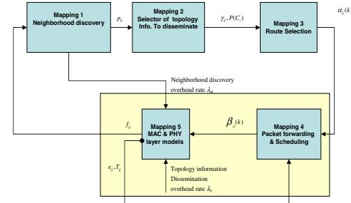
Fig. 1. Architecture of the Component Based Model
