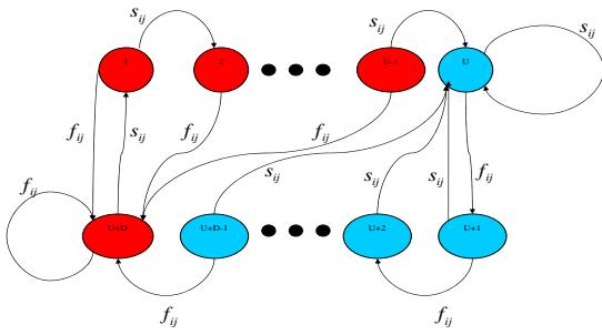
Fig. 2. Markov chain model for the NDC detection mechanism
