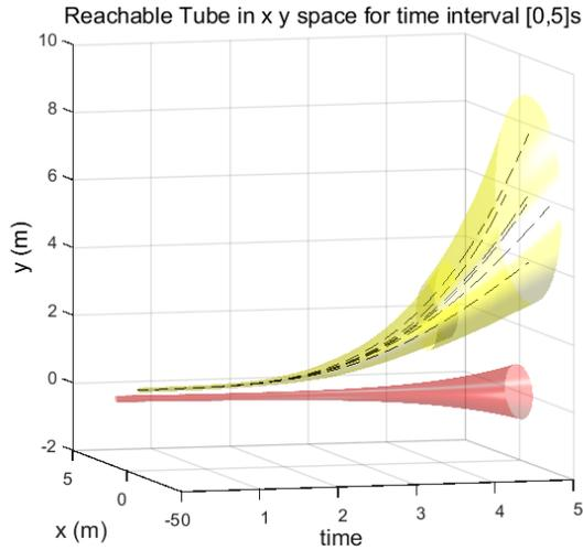
Fig. 2. The reachable tubes for two aircraft after control set design for the first scenario. Clearly, there is no collision between the overapproximation of the reachable tubes. A closer examination also reveals that there is no violation of separation requirement over time. The nonlinear trajectories are within the reachable tube bounds during the whole time horizon.
