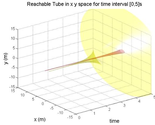
Fig. 1. The initial reachable tubes of both aircraft projected to  $x y$ . The reachable tubes are represented by external approximations computed by Ellipsoid Toolbox. The light yellow tube is the external approximation of the reachable tube of the ego aircraft, while the light red one is the external approximation of the reachable tube of the intruder. Clearly, the reachable tubes collide.
