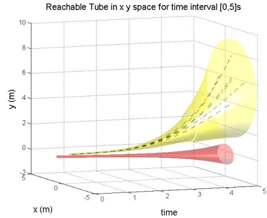
Fig. 3. The reachable tubes for two aircraft after control set design for the second scenario. Since the intruder is moving away, the reachable tube for the ego aircraft is larger in size comparing to the one in Fig. 2. Clearly, there is no collision between the overapproximation of the reachable tubes. A closer examination also reveals that there is no violation of separation requirement over time.
