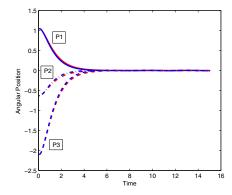
Fig. 2. The red curves show the behavior under continuous feedback and the blue ones for event based feedback. P1, P2 and P3 correspond to pendulum 1, pendulum 2 and pendulum 3 respectively.
