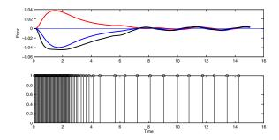
Fig. 3. (upper) The red curve is for the error in angular position of pendulum 1, the blue and black ones are for the same for pendulum 2 and pendulum 3 respectively. (lower) The event triggering profile.
