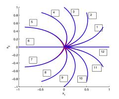
Fig. 4. The red curves are for the continuous feedback system and the blue curves are for the event based system. All the trajectories converge to the equilibrium point at the origin. There are twelve different initial positions as numbered in the figure.
