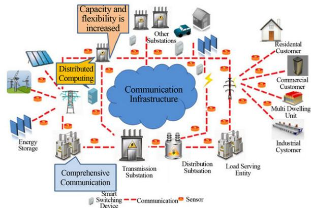
Fig. 1: A Smart-Grid electric network with multiple communication and control sensors.
