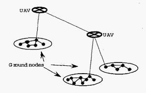
Fig. 1. MANET with three partitions and two connecting UAVs.
